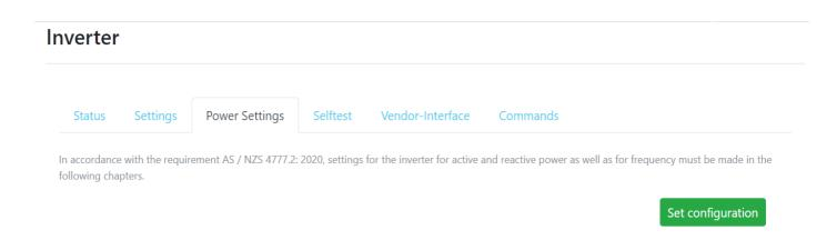
The current grid settings for the sonnenBatterie system will be displayed in this tab, simply scroll down the page to view and confirm with the local DSNP's documentation if needed.
