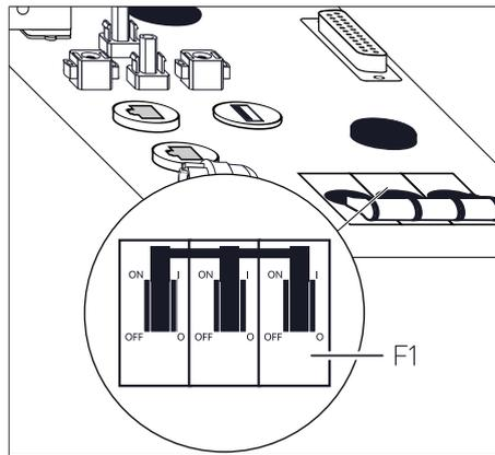
► Switch on fuse switch F1.
