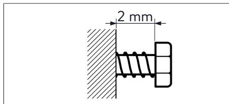
Illustration 12: Distance between screw head and wall
