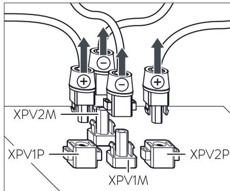
Illustration 62: Removing the PV plug-in connectors
