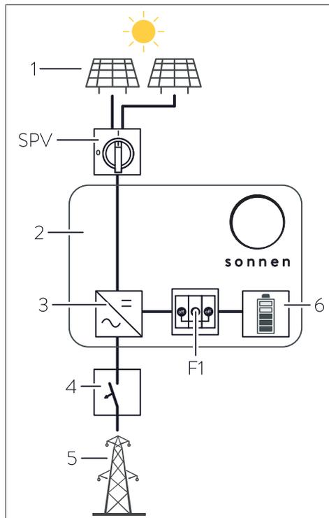
Illustration 2: Block diagram of the switching elements
