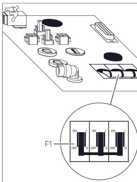
Illustration 61: Fuse switch F1 and PV disconnector
