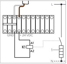
Illustration 43: Activating/deactivating a thermal resistor
