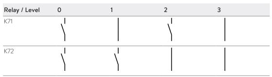
Table 3: Make contact positions of K71 and K72 relays depending on activated level
