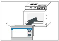
Illustration 27: Inserting the touch display
