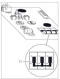
Illustration 61: Fuse switch F1 and PV disconnector
