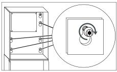
Illustration 16: Tightening the screws
