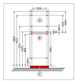
Illustration 10: Drill template for storage system with extension cabinet (figure is not to scale - all specifications are in millimetres)
