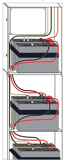
Illustration 53: Connecting the battery lines for up to 15 kWh storage capacity with an extension cabinet
