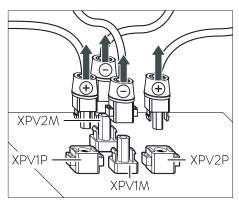
storage system. When doing this, observe the specifications of the connector's manufacturer.
