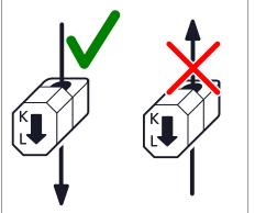
Illustration 23: left: correct energy flow direction / right: incorrect energy flow direction
