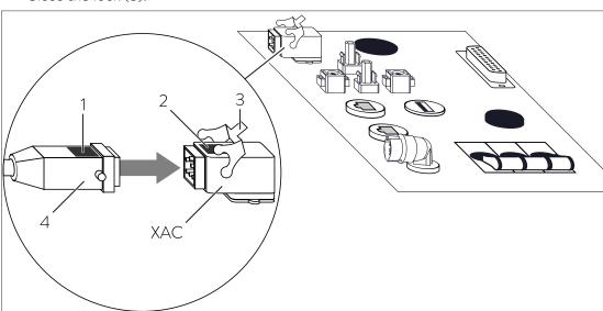
Illustration 37: Connection of the mains line to the connection socket
