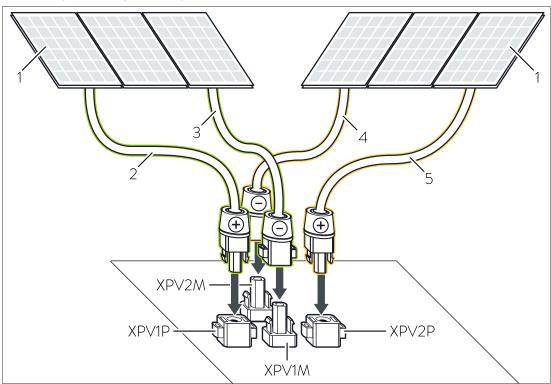
Illustration 57: Connecting the PV system to the storage system
