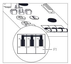
► Switch on fuse switch F1.
