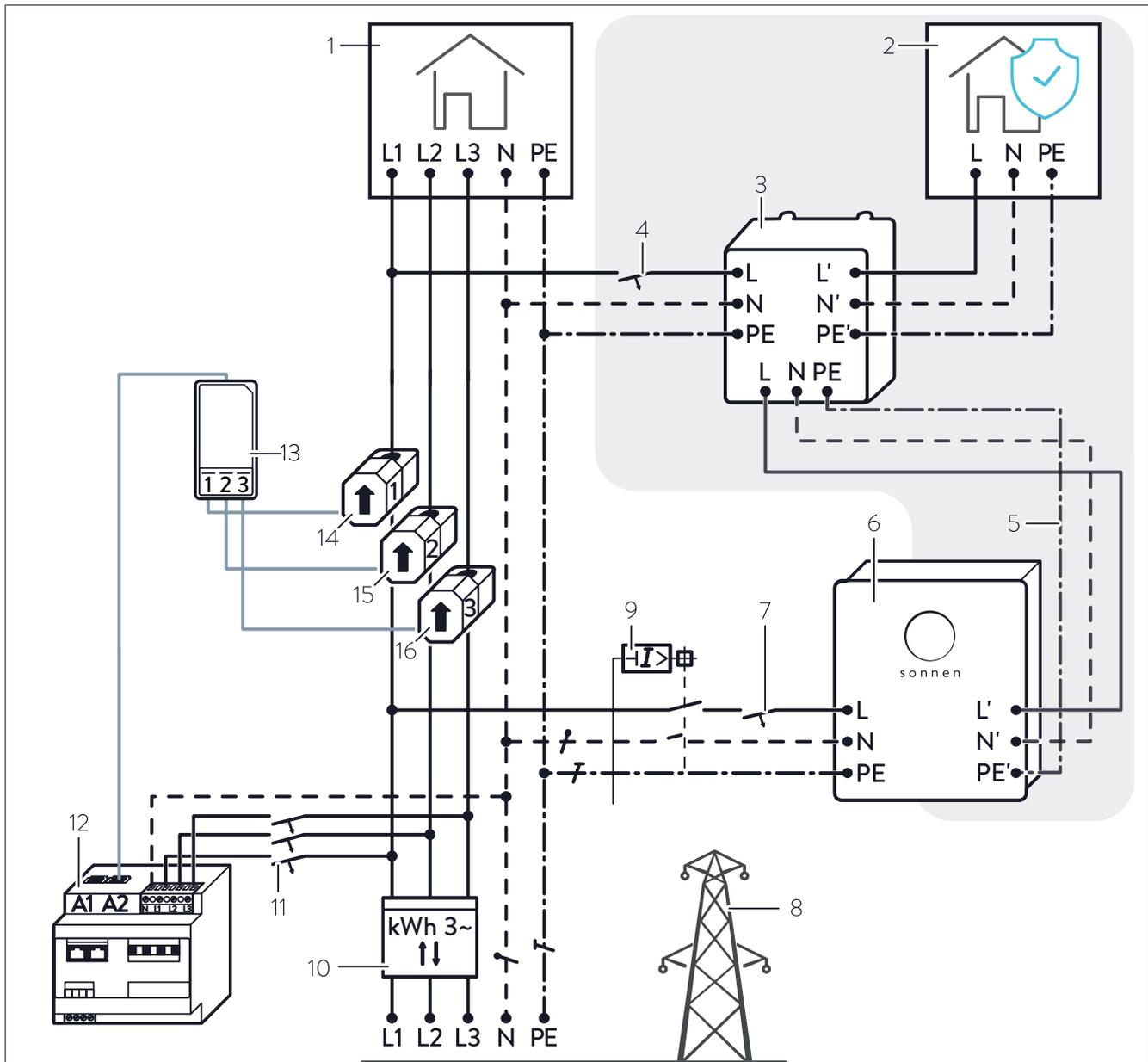
Illustration 5: Circuit diagram overview - electrical connection at three-phase mains
