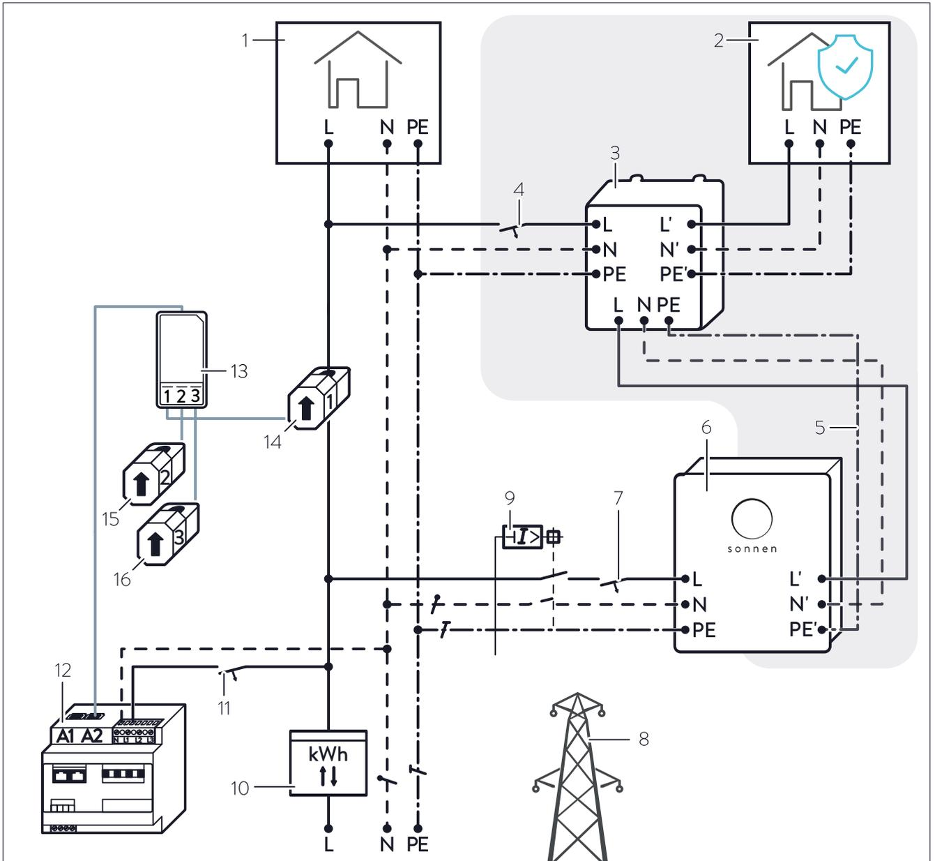
Illustration 4: Circuit diagram overview - electrical connection at single-phase mains
