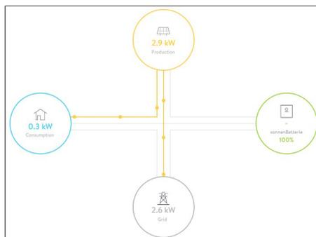
The Live State offers a quick overview of the current distribution of electricity within your household. The different displays are always up-to-date and continuously supplied with live data.
